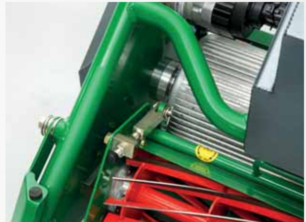
Simple adjustment of cylinder to bottom blade
