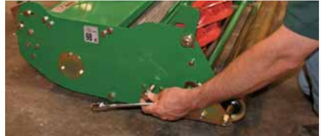
Loosen retaining bolt and slide cassette across
