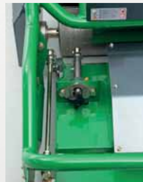
Easy to use click system for height of cut
