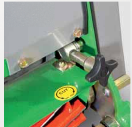
Simple adjustment of cylinder to bottom blade
