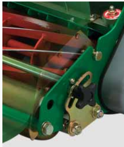
Simple height of cut adjustment
