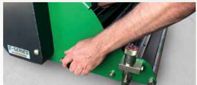
Tighten retaining bolt
