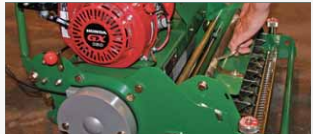
Insert new cassette onto front unit bearing stud
