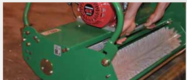
Lower cassette onto back tie bar and slide cassette across
