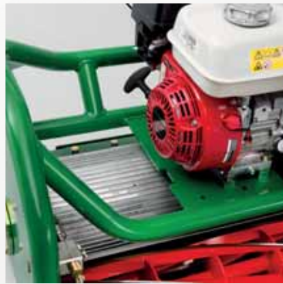
Ribbed rear roller and strong tubular framework
