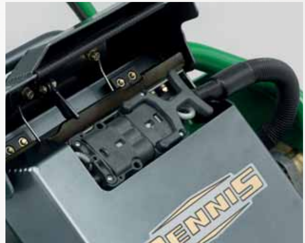
Easy connect/disconnect battery to electrical system
