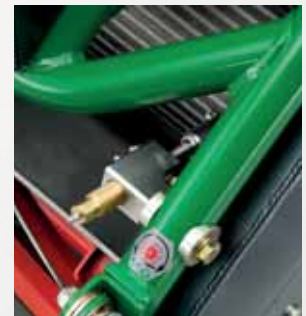
Easy adjustment of bottom blade to cylinder
