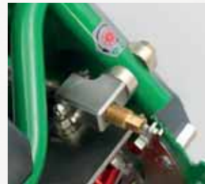
Easy adjustment of bottom blade to cylinder
