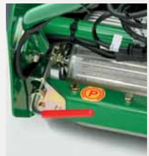
Simple lever operated mechanical parking brake
