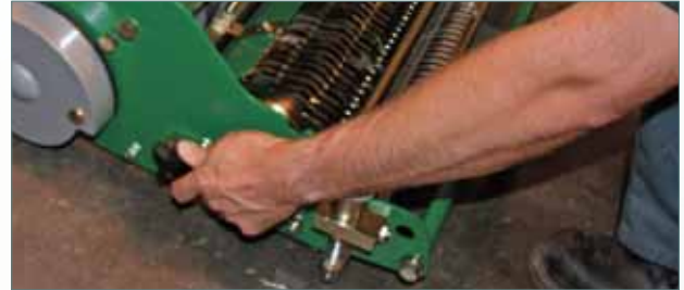
Loosen retaining bolt and slide cassette across
