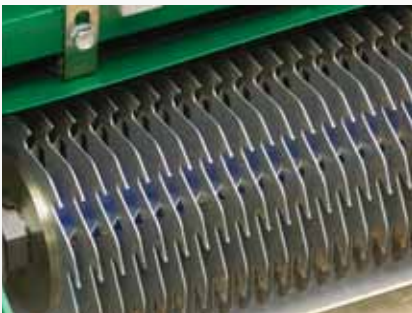
The ultimate verti-cutter with tungsten tipped blades
