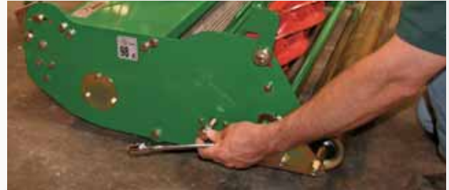
Loosen retaining bolt and slide cassette across
