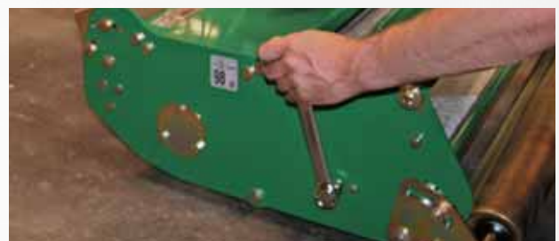
Tighten retaining bolt
