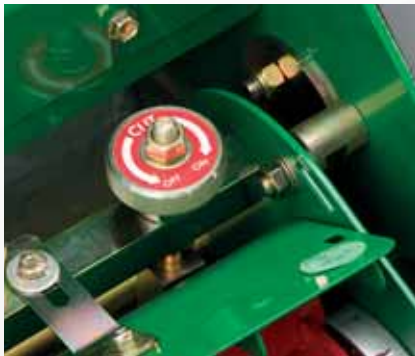
Easy adjustment of bottom blade to cylinder
