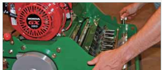
Tighten retaining bolt
