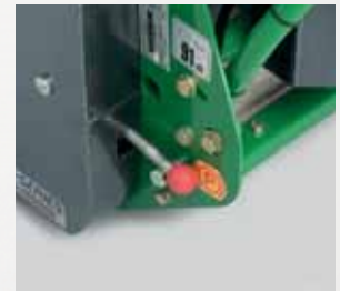
Simple lever operated parking brake
