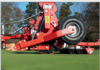
Brush-roller combination for incorporation of top dress material and for smoothing the surface.
