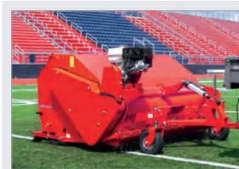
Trailed version for carrier vehicles without rear linkage.
