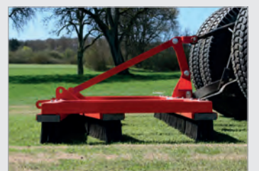
Turf-friendly sand distribution with three rows of brushes with offset alignment.
