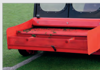
Driven independently from the traction vehicle with the ground-powered design.
