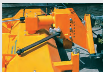
Regular sweeping results with the hydraulic central rotation around the central axis.
