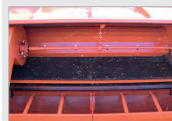
Three-stage cleaning with a coarse riddle screen, fine riddle screen and suction blower.
