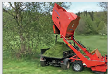
Hydraulic high dumping for easy dumping up to 170 cm.
