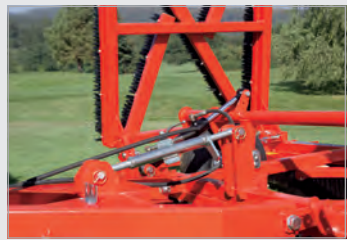
Different sets of brushes with hydraulic lifting and lowering for use on sports grounds, fairways and greens.
